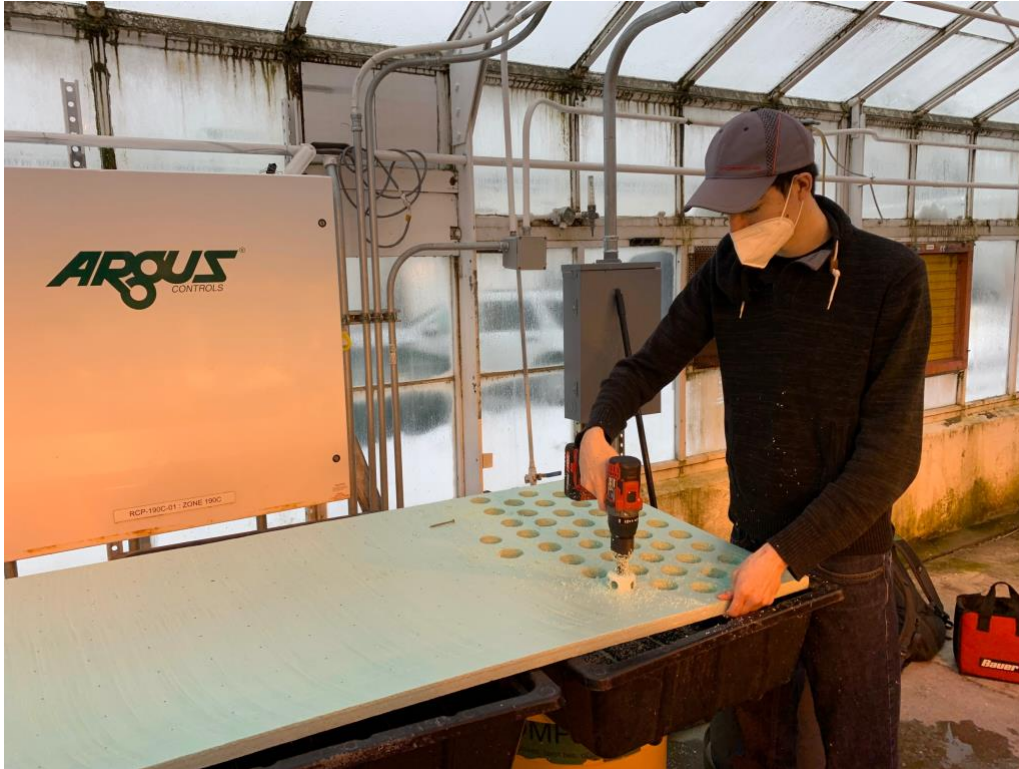
Figure 2: Preparation of 1" thick foam board drilled with 2" holes spaced 3" on center.
