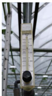
Figure 8. Flow meter for monitoring oxygen addition to ponds.
