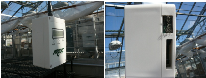
Figure 7. Aspirated box with digital output screen in greenhouse (left). The picture on the right shows the opening for the box that allows the fan in the bottom of the box to draw air over the sensors for a more accurate temperature reading.
