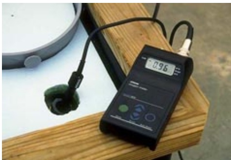
Figure 10. Dissolved oxygen sensor. DO levels should be greater than 4 ppm to prevent growth inhibition. Visible signs of stress may be observed at 3 ppm.
