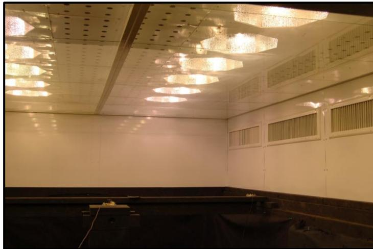
Fig. 1. Growth chamber with Cycloptics luminaires; black cloth, side rails and crossbar in place; and showing the reference light sensor position.
