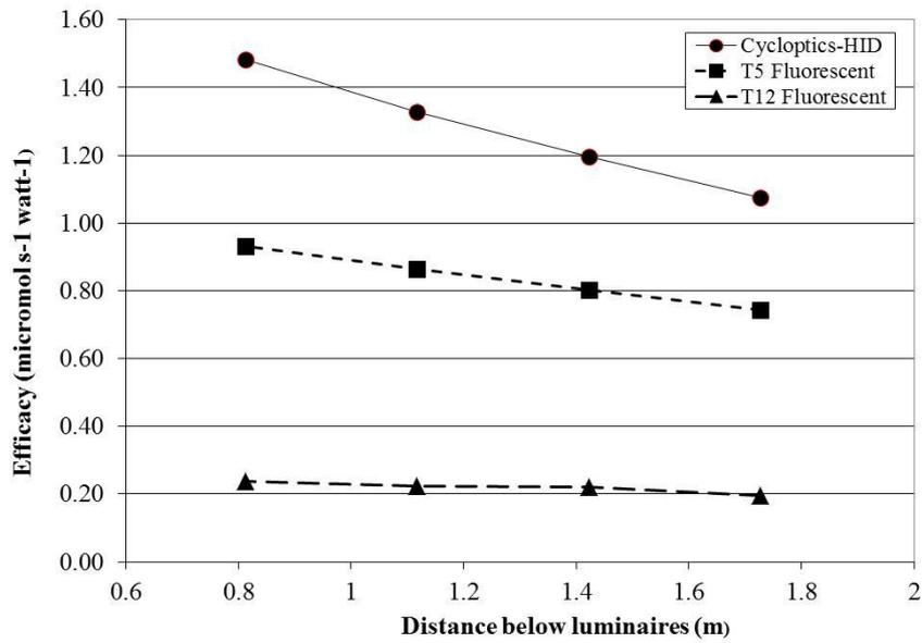
Fig. 2. Average efficacy of light delivery by three chamber lighting systems. Data determined for one quadrant, n = 24, using platform method
