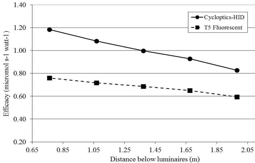
Fig. 1. T5 fluorescent compared to Cycloptics HID, in efficacy of light delivery to five planes below the luminaires. Data determined for chamber, n = 96.
